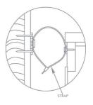
3. Move the furniture to its final position and alian the bracket on the furniture with the bracket on the wall. Thread the strap through the bracket as shown, and tighten until snug. Do not over-tighten.
